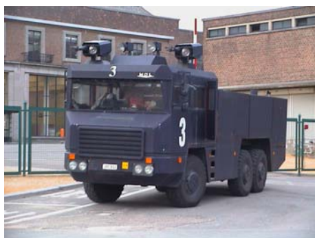
FIGURE 3: A typical vehicle mounted water cannon
